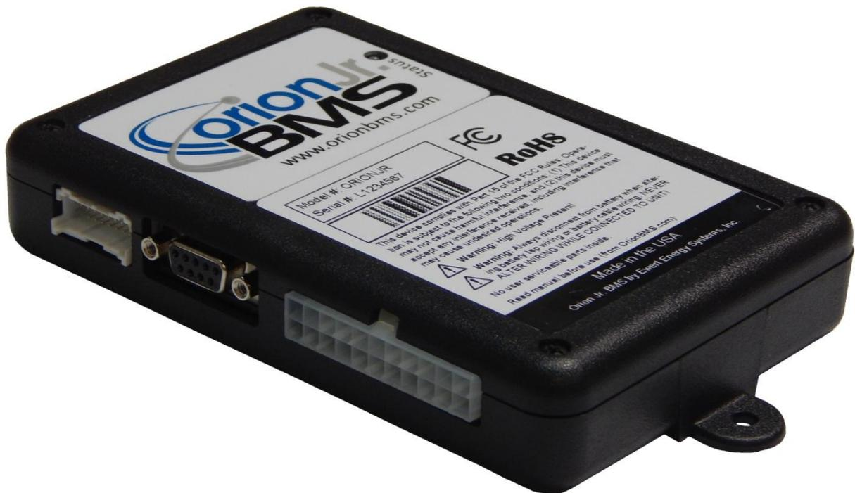
The Orion Jr. BMS by Ewert Energy Systems is designed to manage and protect Lithium ion battery packs and is suitable for use in stationary energy storage and small mobile applications such as golf carts and material handling equipment.
